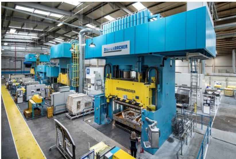
Figure 2 - Creative Composite's range of SMC Presses (can deliver up to 3000T pressure)
